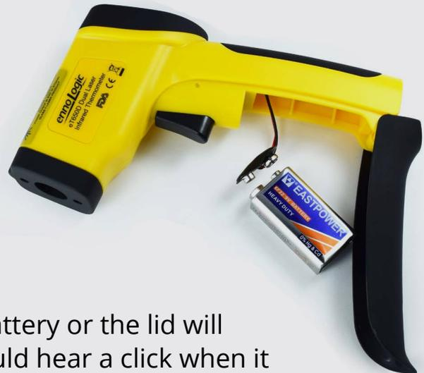
Be sure to tuck the wires in next to the battery or the lid will not close properly. Close the lid. You should hear a click when it snaps into place.
