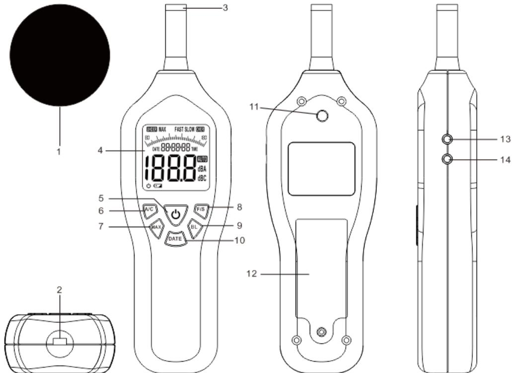
1. Foam ball microphone cover (mandatory for outdoor use to prevent wind noise from affecting the measurement)
