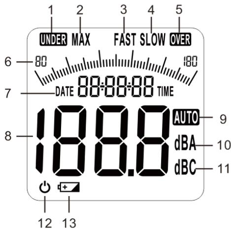
1. **UNDER:** Under-range alert symbol, will be displayed if the reading is below the lowest detectable sound level.
