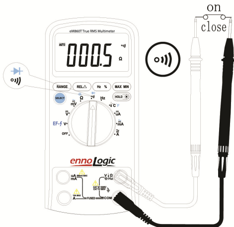
Figure 3-4a: Checking Continuity - Short
